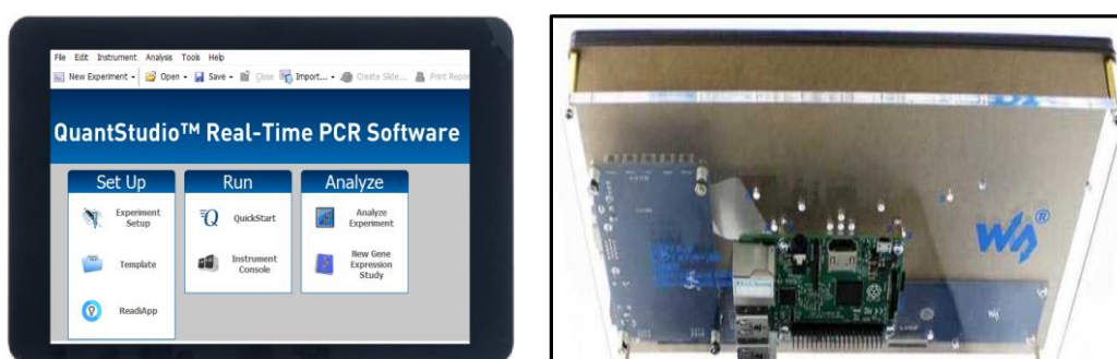
Figure 3. The control screen of PCR software and back side seen mounted PC-main board for 10.1-inch LCD touch screen [13].
